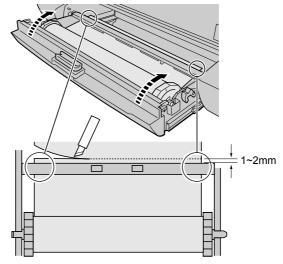
**10** After closing the roll media tray, close the tray. Firmly push the roll media tray completely into the printer.
